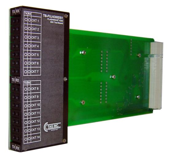
The TB-FUJ4300DS1 provides a quick method to transmit an acceptable test signal from the FLASHWAVE 4300 DS1 card slots to the DSX-1. At the DSX-1, Tester 2 will loop the signal back to the TB-FUJ4300DS1 and determine if the signal is acceptable for system turn up. The wiring label indicates Transmit (Tx) and Receive (Rx) bantam jacks for the 14 DS1 circuits. The TB-FUJ4500DS1 is used on non-powered systems.
