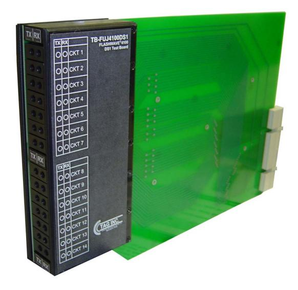
The TB-FUJ4100DS1 provides a quick method to transmit an acceptable test signal from the FLASHWAVE 4100 DS1 card slots to the DSX-1. At the DSX-1, Tester 2 will loop the signal back to the TB-FUJ4100DS1 and determine if the signal is acceptable for system turn up. The wiring label indicates Transmit (Tx) and Receive (Rx) bantam jacks for the 14 DS1 circuits. The TB-FUJ4100DS1 is used on non-powered systems.
