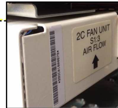
2C FAN TRAY UNIT (SIDE VIEW)
