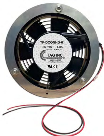
PN # TF-DCONHD-01 48 Volt Replacement Fan for DCO Non High Density CMF Bay w/ 2 Wire Open End (for splicing) (Black -48V, Red +48 Return) Includes: Guard Grill & (1) Butt Splice
