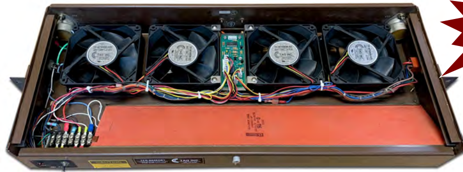
REFURBISHED DMS OPM, NT8X06AB FAN TRAY * WITH (4) NEW 48V FANS & NEW ALARM CONTROL BOARD
