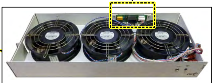
LUCENT 2B FAN TRAY w/ (3) EXISTING FANS (BOTTOM VIEW) (fan tray is not included)
