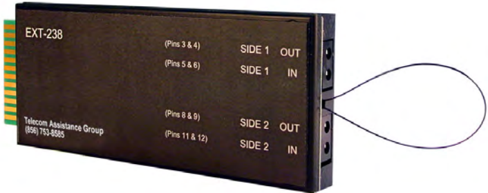
(1) # EXT-238 T1 Line Repeater Access Board
