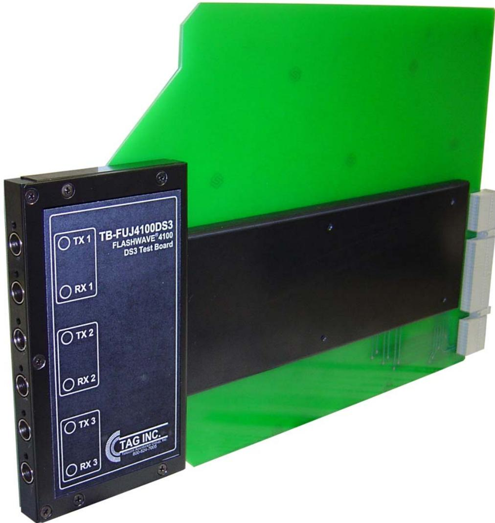
The TB-FUJ4100DS3 provides a quick method to transmit an acceptable test signal from the FLASHWAVE 4100 DS3 card slots to the DSX-3. At the DSX-3, Tester 2 will loop the signal back to the TB-FUJ4100DS3 and determine if the signal is acceptable for system turnup. The wiring label indicates Transmit (Tx) and Receive (Rx) 440A jacks for the 3 DS3 circuits. The TB-FUJ4500DS3 is used on non-powered systems.
