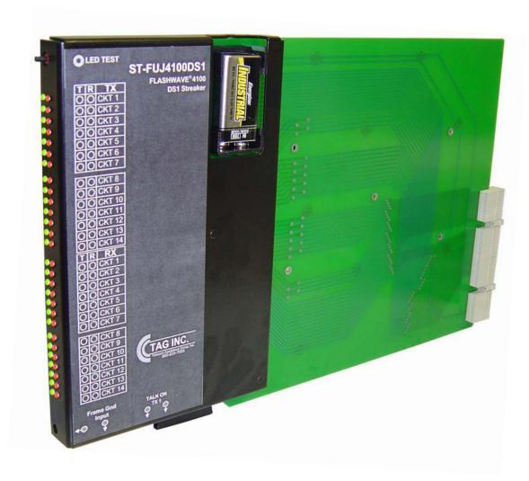
The ST-FUJ4100DS1 provides a quick method to verify wiring continuity "streak" from the FLASHWAVE 4100 DS1 card slots to the DSX-1. At the DSX-1, Tester 2 will ground the connection point and the ST-FUJ4100DS1 will light the LED associated with that connection. The wiring label indicates LED's for 14 DS1 circuits. The ST-FUJ4100DS1 is powered by a 9-Volt battery.
