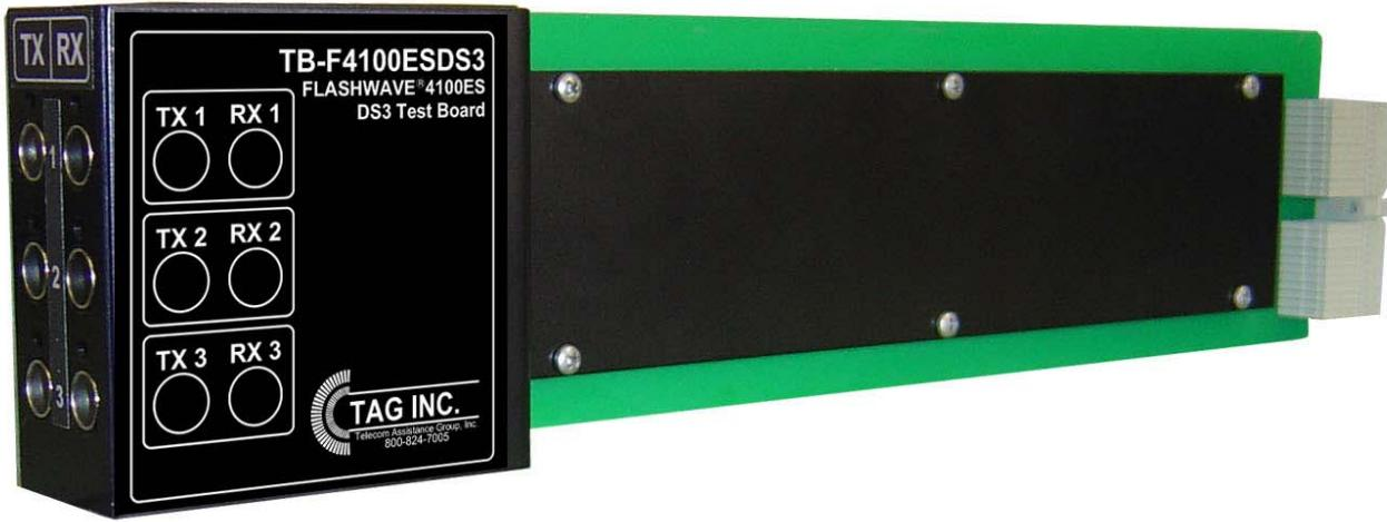
The TB-F4100ESDS3 provides a quick method to transmit an acceptable test signal from the FLASHWAVE 4100ES DS3 card slots to the DSX-3. At the DSX-3, Tester 2 will loop the signal back to the TB-F4100ESDS3 and determine if the signal is acceptable for system turnup. The wiring label indicates Transmit (Tx) and Receive (Rx) 440A jacks for the 3 DS3 circuits. The TB-F4100ESDS3 is used on non-powered systems.
