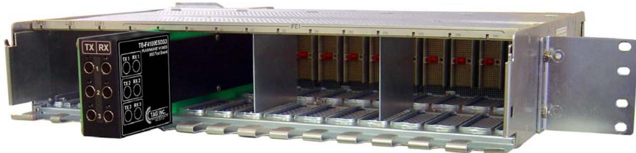
\*The (TB-F4100ESDS3) FLASHWAVE\* 4100ES DS3 Test Board will plug into slots 3-14
