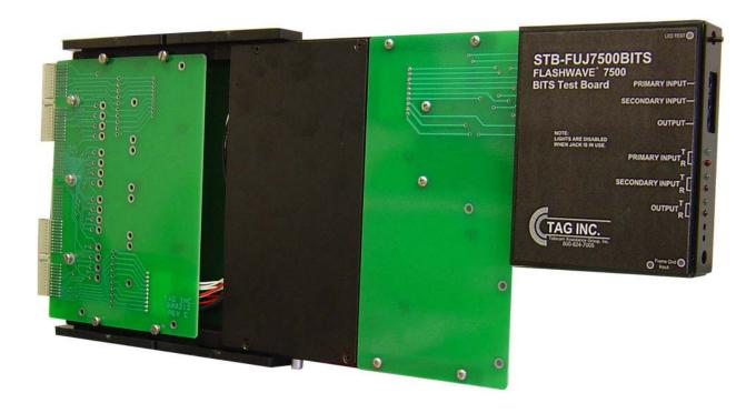
The STB-FUJ7500BITS provides a quick method to verify continuity as well as, transmit a test signal from the FLASHWAVE 7500 BITS card slots to the DSX-1. At the DSX-1, Tester 2 will use a continuity test probe to verify that the BITS card slot is properly wired. Tester 2 is also capable of looping a test signal back to the STB-FUJ7500BITS and Tester 1 can determine if the signal is acceptable for system turnup. The STB-FUJ7500BITS is used on non-powered systems.
