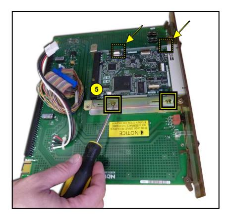
5. Remove the (4) screws & washers attaching the OLD drive to the mounting rails on the circuit pack.
