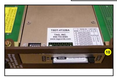
**10.** Position the TSDT-4T32BA flush with the cutout of the faceplate on the circuit pack as shown.
