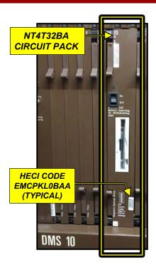
The procedure on the following pages details removing mechanical Magneto-Optical (MO) drives on DMS10 NT4T32BA circuit packs & replacing them with a <u>NEW</u> TAG Solid State SCSI Drive (PN # TSDT-4T32BA).
