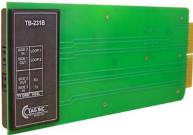
TB-231B 220 (Kentrox size) Office Repeater Test Board w/ Bantam Jacks 12 STATE SOUTHEAST ATT.100071973 ATT.100001307
