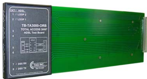
TB-TA3000-ORB Adtran Total Access 3000 Test Board w/ Bantam Jacks
