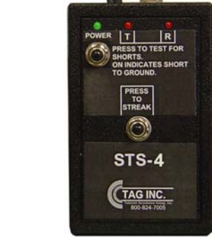
(1) STS-4 Streaker Test Sender Unit (required to streak)
