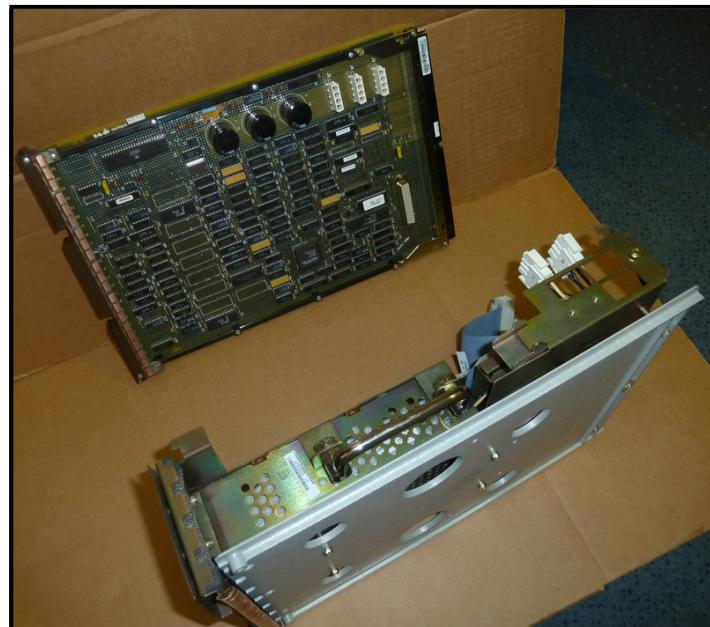
6. Place the circuit pack down on an anti-static surface.
