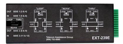
Plugs into T1, 56KB, HDSL, ISDN Apparatus Cases
