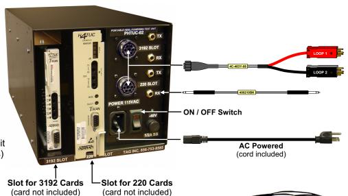
(1) # PHTUC02 Portable HDSL Powering / Test Unit (3192 & 220 Cards)
