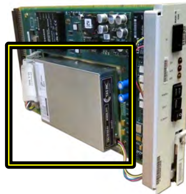
NEW HARD DRIVE (installed on UN375E/F circuit pack)
