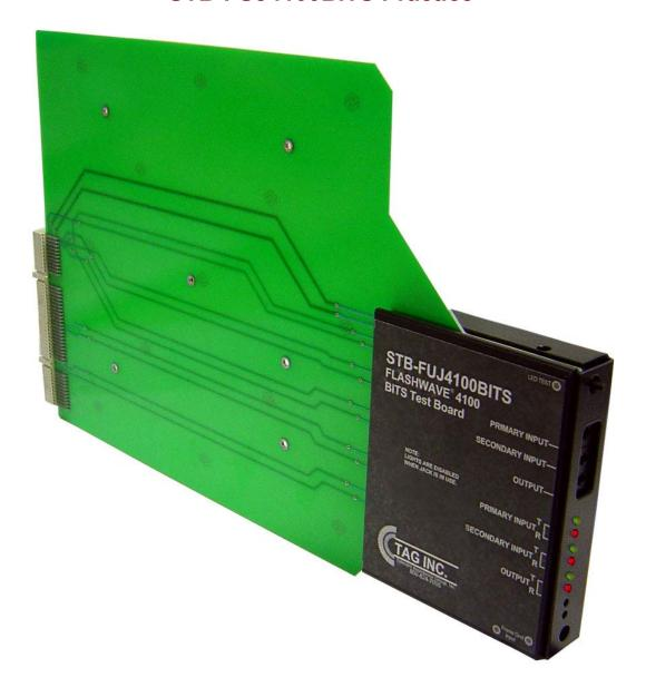
The STB-FUJ4100BITS provides a quick method to verify continuity, as well as, transmit a test signal from the FLASHWAVE 4100 BITS card slots to the DSX-1. At the DSX-1, Tester 2 will use a continuity test probe to verify that the BITS card slot is properly wired. Tester 2 is also capable of looping a test signal back to the STB-FUJ4100BITS and Tester 1 can determine if the signal is acceptable for system turn up. The STB-FUJ4100BITS is used on non-powered systems.
