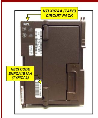
The procedure on the following pages details removing a **DAT Tape Drive** from a **DMS-100, XA-CORE NTLX07AA** circuit pack & replacing it with a **NEW** TAG Solid State SCSI Drive (#TSDT-NTLX07-01).
