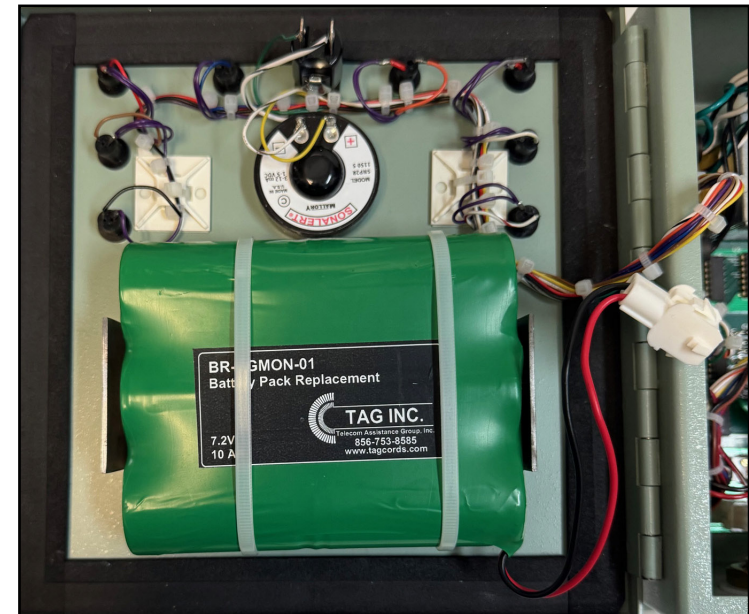
INSIDE VIEW of NEW NIMH BATTERY PACK 7.2V, 10Ah 72Wh,3X
