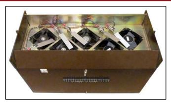
NORTEL NT3X90AA / NT3X90AB, DMS-100 SWITCH BAY (AC POWERED) w/ EXISTING FANS (5 FANS PER TRAY)
