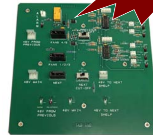
Fan Control Board w/ built in Sensors (no paddles needed)
