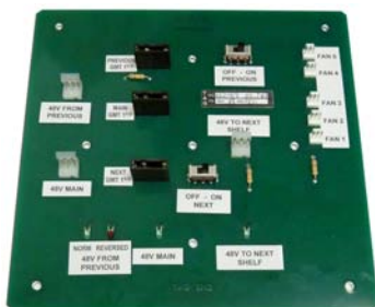
(1) Fan Control Board w/ Cabling & Mounting Hardware
