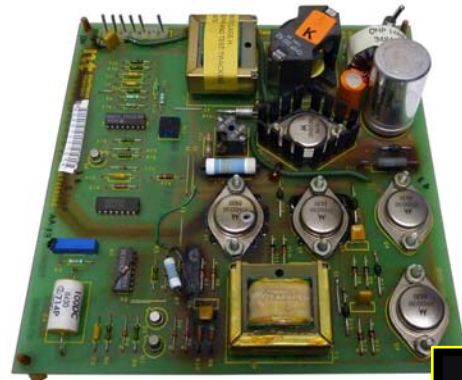
BURNED OUT 24VAC CIRCUIT BOARD
